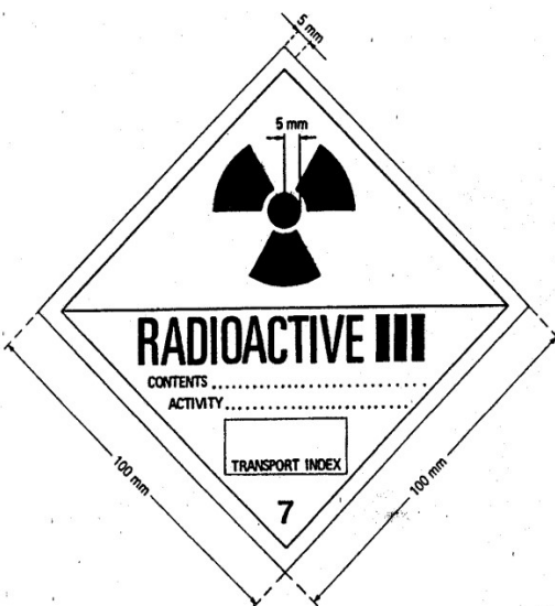
Fig 4: Category III-YELLOW label. The background colour of the upper half of the label shall be yellow and of the lower half white, the colour of the trefoil and the printing shall be black, and the colour of the category bars shall be red.
